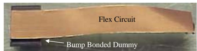
Figure 9: Dummy Bump Bond Structure
